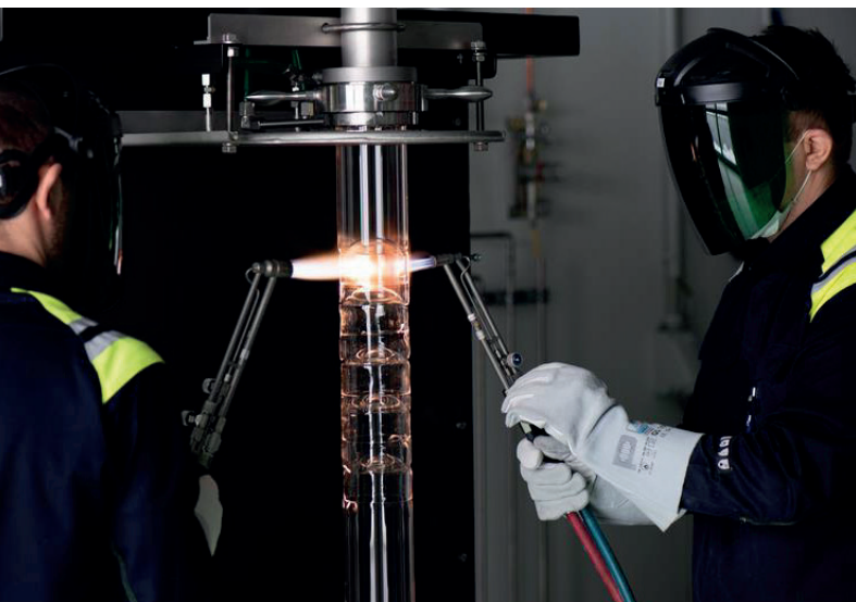
The crystals required for the photon counters are grown in ampoules which technicians elaborately seal at 3,000°C. Source: Siemens Healthineers
